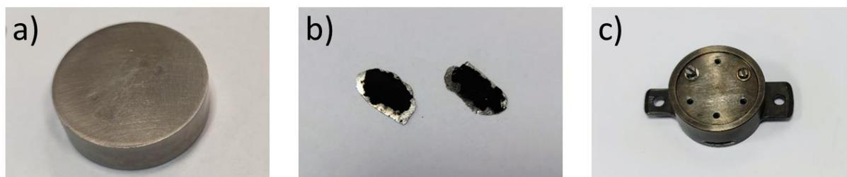
Figure 17 A steel roller a), an exemplary sample pressed into an indium piece b), a molybdenum holder c).
