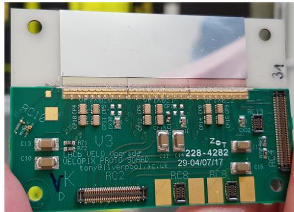
**Figure 3.21:** The VeloPix ASIC at the final stage of development.
