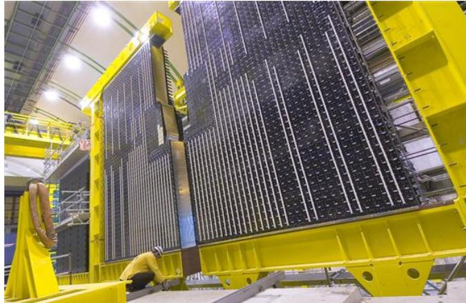
**Figure 3.7:** The LHCb electromagnetic calorimeter ECAL. [257]
